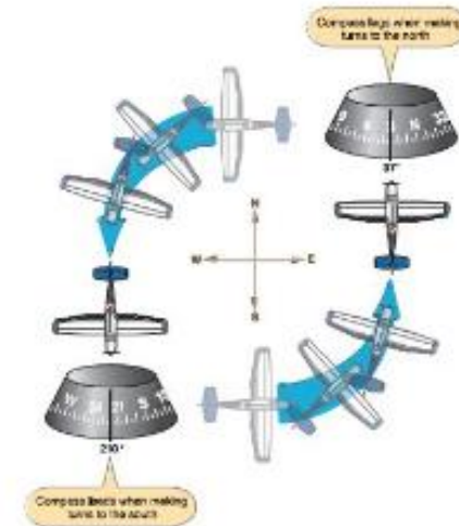
Figure 7-35. North and south turn error.
